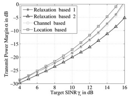
Fig. 2 Average transmit power margin  $\alpha$  to the power limit at each BS against the target SINR  $\gamma_i$ 's at MSs
