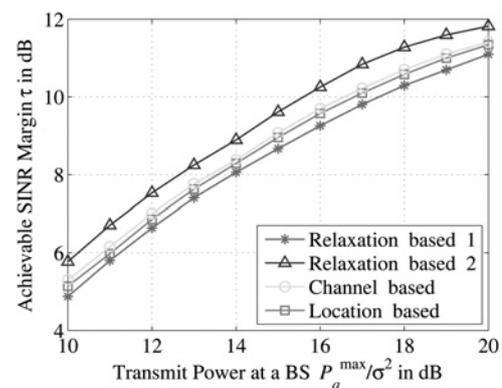
Fig. 3 Achievable SINR margin  $\tau$  at the MS against the power constraints at each BS
