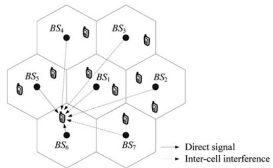
Fig. 1 Seven-cell network with ten randomly located mobile stations
