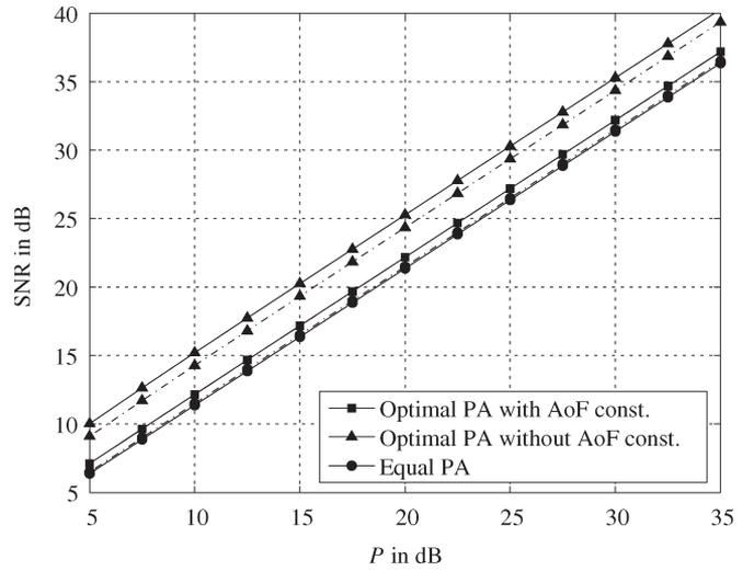
Fig. 7. Effective average SNR at the destination with different PA schemes. ("Dash-dot" lines) Exact SNR. (Solid lines) SNR evaluated by (8).
