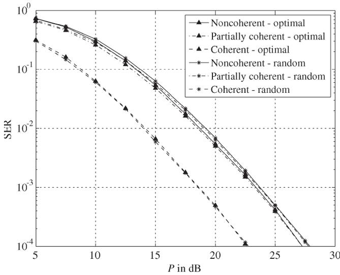
Fig. 5. Symbol error performances of the proposed DUSTM and a random code with  $\sigma_F^2 = 1$  and  $\sigma_G^2 = 10$ .
