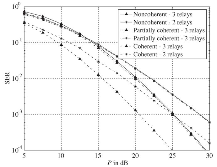
Fig. 4. Symbol error performance of DUSTM with  $\sigma_F^2 = 1$  and  $\sigma_G^2 = 10$ .
