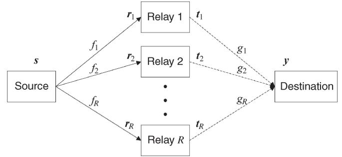
Fig. 1. Block diagram of distributed space–time modulation in a wireless relay network with  $R + 2$  nodes.
