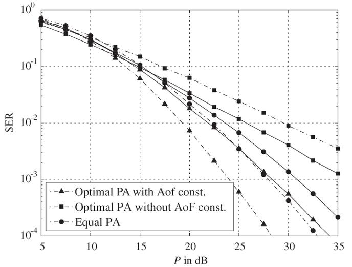
Fig. 8. Performance of noncoherent DUSTM with different PA schemes. ("Dash-dot" lines) Three-relay system. (Solid lines) Two-relay system.
