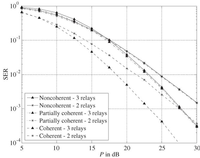
Fig. 2. Symbol error performance of DUSTM with  $\sigma_F^2 = 1$  and  $\sigma_G^2 = 1$ .
