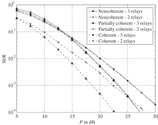
Fig. 3. Symbol error performance of DUSTM with  $\sigma_F^2 = 10$  and  $\sigma_G^2 = 1$ .
