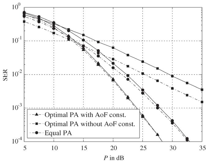
Fig. 9. Performance of DUSTM for a three-relay network with different types of detections and PA schemes. (“Dash-dot” lines) Partially coherent detections. (Solid lines) Noncoherent detections.
