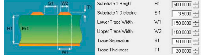
Fig. 4. Differential microstrip stackup &amp; dimensions (in microns).
