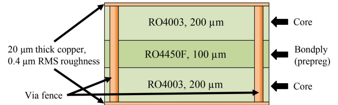
Fig. 6. Stack-up of 200 \mu\text{m} of RO4003, 100 \mu\text{m} of RO4450F, and 200 \mu\text{m} of RO4003 for a combined height of 500 \mu\text{m} .
