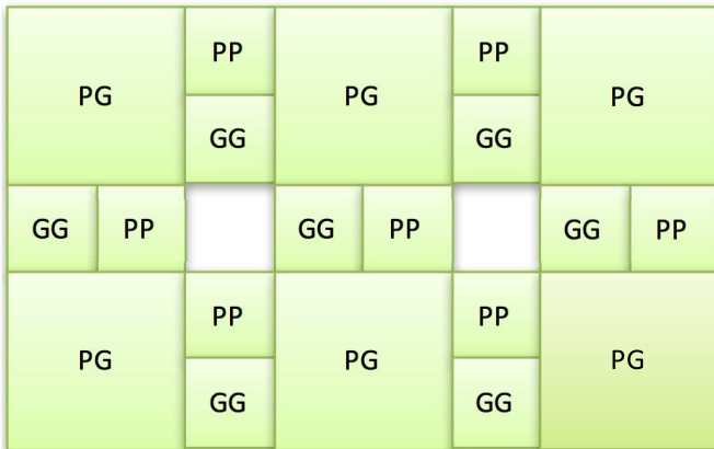
Fig. 2. Example layout with 3 \times 2 PG segments that would be interconnected with low IR -drop, but isolated from each other at high frequencies due to PP and GG segments.
