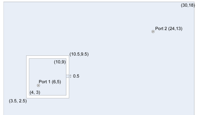
Fig. 7. Geometry of the power island and the bridge with a width of 0.5 mm connected to the center of the power island’s right edge. All units are in millimeters.
