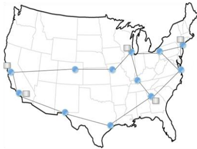
Figure 1: Network Topology; squares=datacenters, circles = routers
