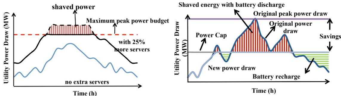
Figure 1. Sample peak shaving a) with and b) without extra servers [10]
