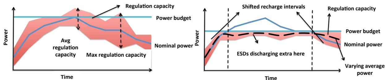
Figure 3. Regulation using ESDs, with i) flexible and ii) fixed power budget
