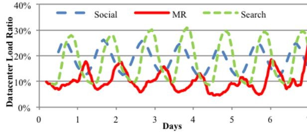
Fig. 4 Sample datacenter load ratio with different job types
